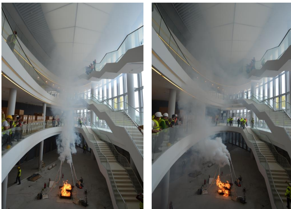
Fig. 6 Smoke plume in an atrium before (left) and after (right) a mechanical smoke extract system is turned on. Visible distortion of the plume by excessive velocity of replacement air coming from one direction.
