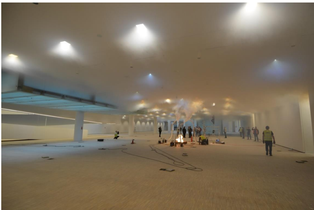
Fig. 5 Hot smoke test in an exhibition hall (mechanical ventilation)
