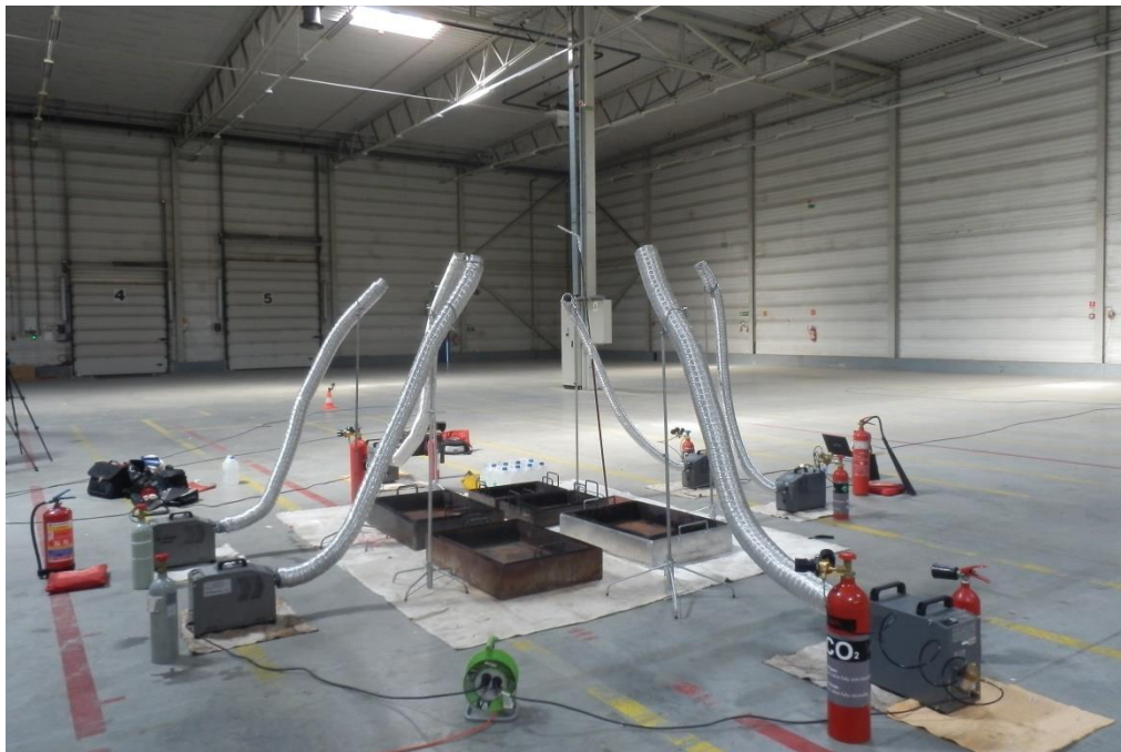
Fig. 1 Example of a test set up for a hot smoke test in a warehouse with 1.5 MW test fire
