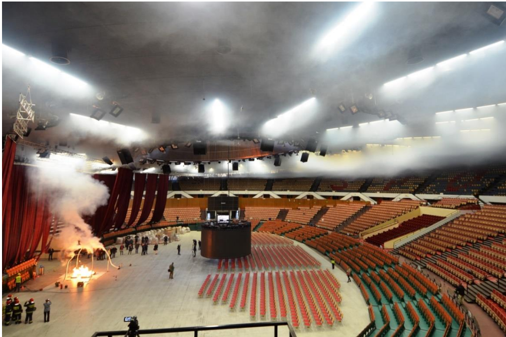
Fig. 4 Hot smoke test in a multi-purpose hall (natural ventilation)
