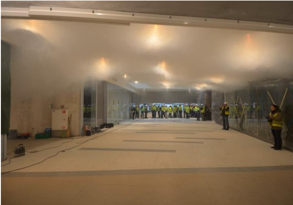
Fig. 2 Flowing hot smoke layer in a shopping mall (test fire in the adjacent retail unit)
