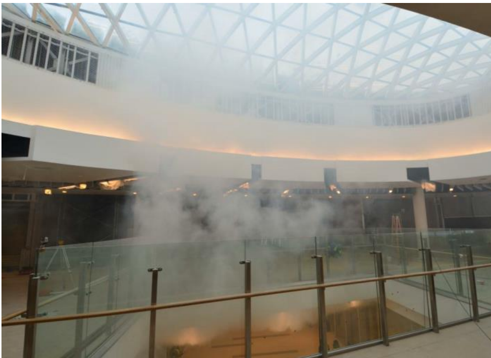
Fig. 3 Spill plume at the edge of floor void in a two storey section of a shopping mall
